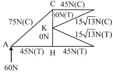
$$(A) S_a = 75 \text{ N(C)} \text{, } S_b = 45 \text{ N(T)}$$
