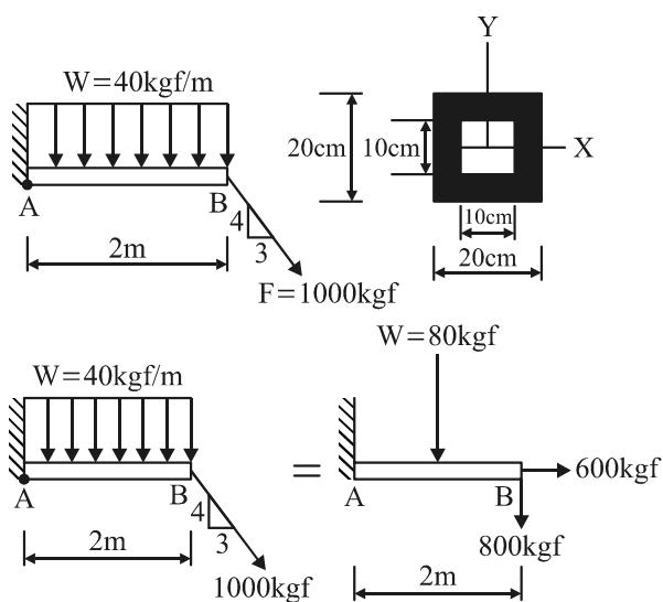
$$M_A = 40 \times 2 \times 100 + 800 \times 200 = 168000 \text{ kgf-cm} \quad (\text{clockwise})$$
