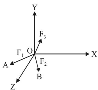
$$\begin{aligned} F_1 &= (-3, 2, 6), F_2 = (2, -4, 4), F_3 = (F_{3X}, F_{3Y}, F_{3Z}) \\ + \rightarrow \sum F_x &= 0 \end{aligned}$$
